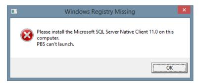
You will find a 32 bit and 64 bit install of Native Client 11.0 in the PBS top-level folder called *Native Client11.0*. Select either the 32 bit or 64 bit version and install it before you continue.
