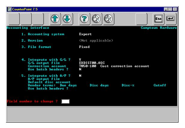
The only fields that can differ from above screen are "G/L Output file" and "Correction Account", both under # 4. (Note: If you are using the A/P interface, field #5 may differ from the above example)
